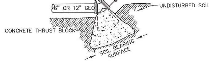
ELBOW - ELEVATION VIEW
