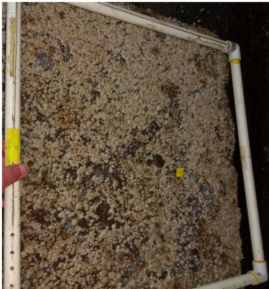
Figure 2. Photo quadrats taken from the Ocean Sentinel anchors after over two years of deployment. The photo on the left is a side of the anchor and the photo on the right is the top of the same anchor.
