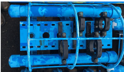
Figure 6: CSM Sub-surface plates. 4 per turn (usually). 3'x2'
