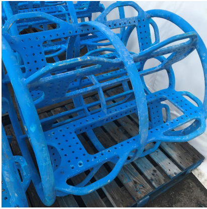
Figure 3: Near-surface Instrument Frames. 6 per turn. 3' diameter x 3' tall.
