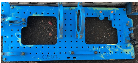
Figure 6: CSM Sub-surface plates. 4 per turn (usually). 3'x2'
