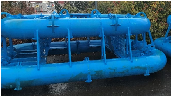
Figure 4: Multifunction Node (MFN). 2 per turn. ~2000# 8'x6'x3' tall.
