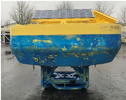
Figure 1: Coastal Surface Mooring (CSM). 4 per turn. Foam disc is 10' diameter, aluminum structure is ~2'. ~3000# as shown, buoys will be delivered without the shown solar panels. There is a 4'x4' interior space in the disc that needs painted.
