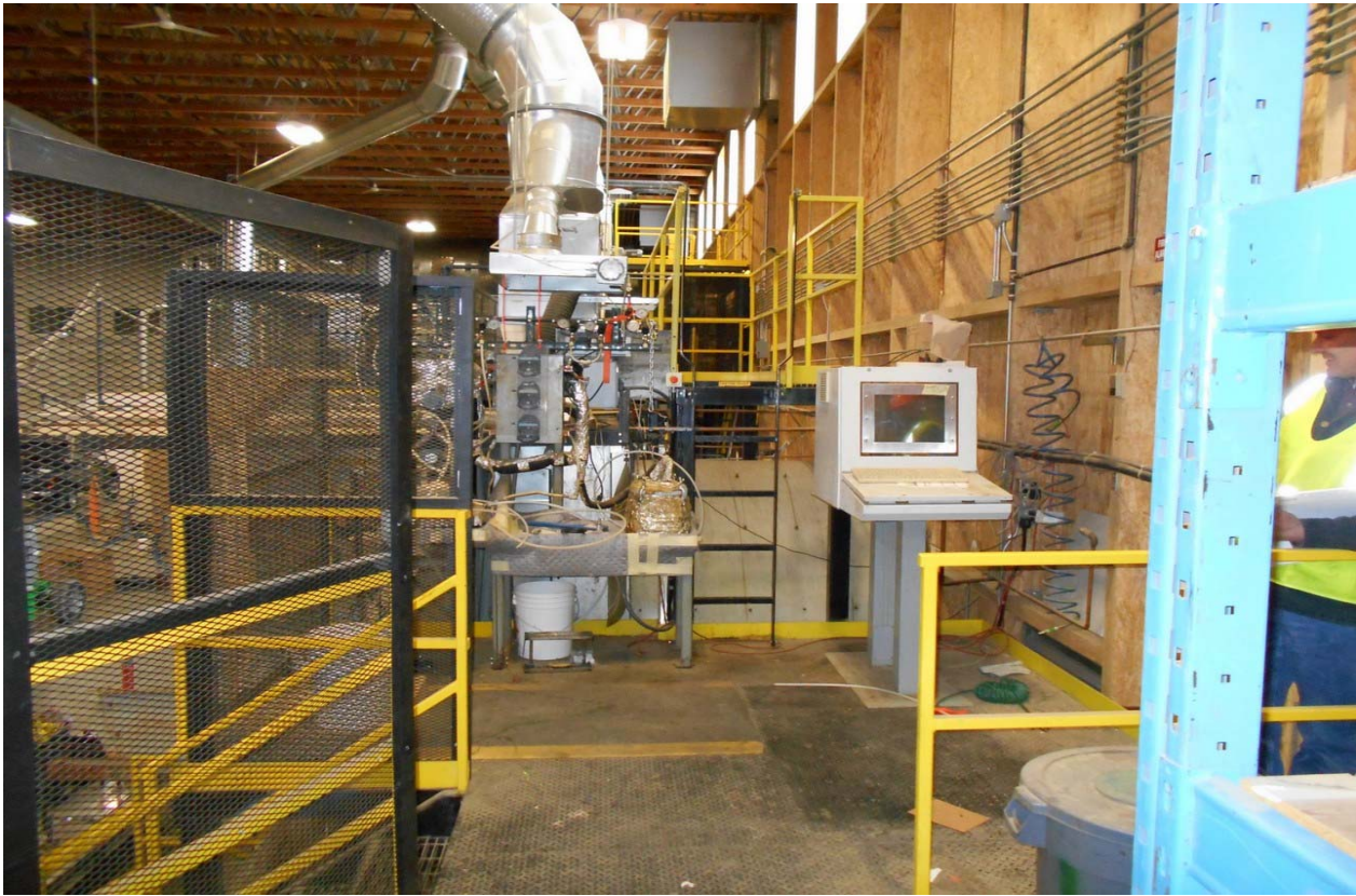
Resin blender access catwalk and stairs approximate shipping dimensions; 12' x 16' x 10' and 8' x 8' x 12', 4,000#
