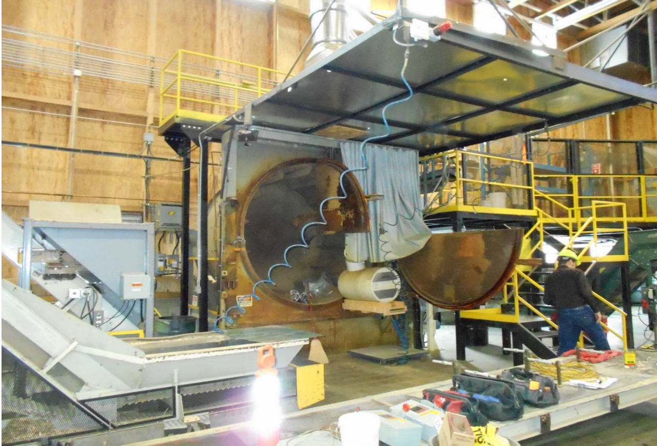
Resin blender drum mount frame, approximate shipping dimensions; 8' x 11' x 15', 3,000#
