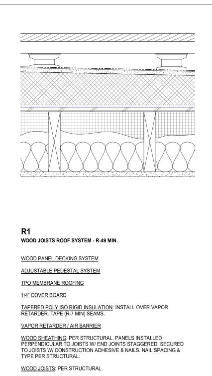
SPRAYFOAM & BATT INSULATION: APPLY 3" MINIMUM THICK (R-21) LAYER SPRAYFOAM TO UNDERSIDE OF SHEATHING BETWEEN JOISTS. FILL REMAINING CAVITY W/ (R-21) BATT INSULATION. (1) LAYER 5/8" GWB: APPLIED AT RIGHT ANGLES TO JOISTS, 24" O.C., WITH 1 1/4" TYPE S OR TYPE W DRYWALL SCREWS 24" O.C.
