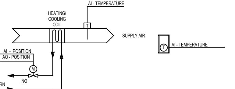
HEATING HOT WATER COIL SEQUENCE OF OPERATION
