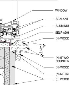
SEALANT ALUMINIUM ANGLE SELF-ADHERED MEMBRANE FLASHING (N) WOOD SILL
