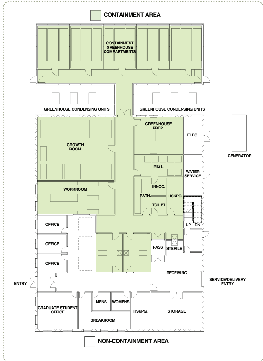
FIGURE 7. Typical Containment Facility Floor Plan*
