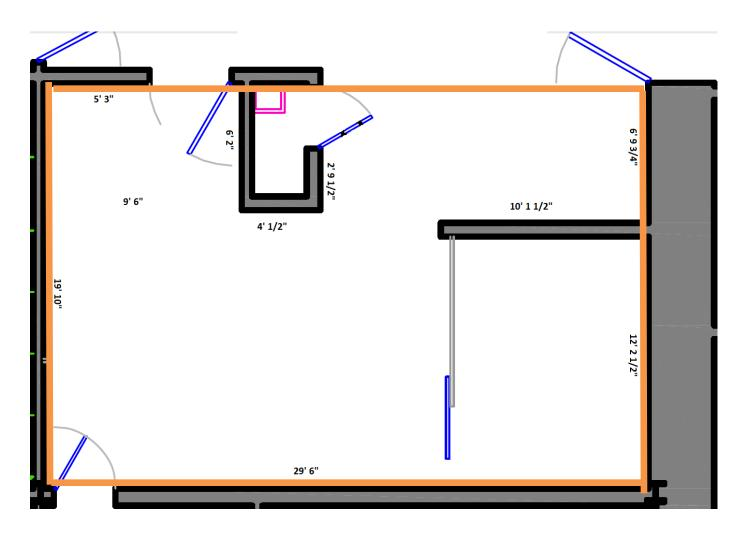
Proposer must verify (based on the floor plan above) that the equipment being proposed will fit in the space and be able to be delivered into the building to the final space, as indicated on the Routing Floor Plan (based on floor plan below)
