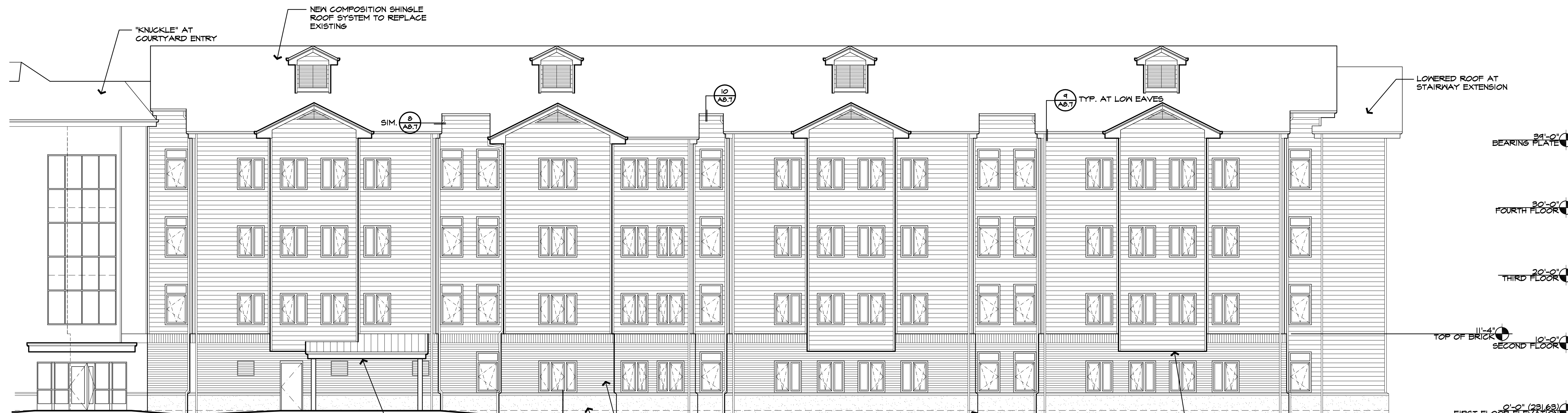
3 COURTYARD ELEVATION - EAST SCALE: 1/8" = 1'-0"
