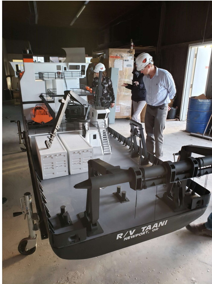
Figure 16 RCRV shipyard supplied 1/10 th scale physical model
