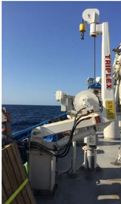
275 Figure 14 Example davit B, can act as core stand when stowed at Position 1
