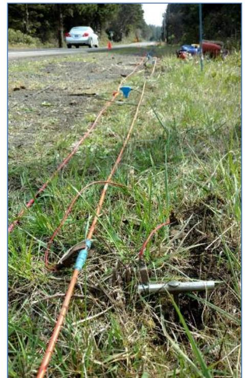
(tomogram). In this case, SA used the Dipole-Dipole array with electrode spacing of either 4 or 6.25 m. Electrode pins were 20 inch long, 3/8 inch diameter stainless rods fully embedded into mineral earth and wetted with a saline solution to reduce contact resistance.
