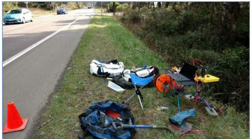
and marine soil, and rock properties that are very difficult to obtain through alternative methods. SA recorded passive ambient vibrations (background noise) augmented by an active, un-timed seismic source (plate and hammer) operated along the array to induce higher frequency, rapidly attenuating energy.
