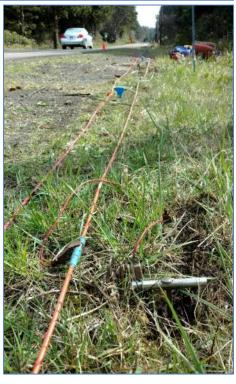
(tomogram). In this case, SA used the Dipole-Dipole array with electrode spacing of either 4 or 6.25 m. Electrode pins were 20 inch long, 3/8 inch diameter stainless rods fully embedded into mineral earth and wetted with a saline solution to reduce contact resistance.
