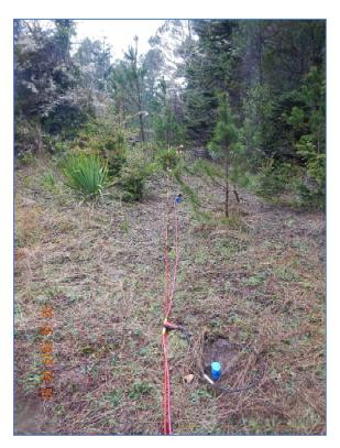
Data were recorded using a networked pair of DAQ 4 seismographs manufactured by Seismic Source in Ponca City, Oklahoma, USA, connected to an IBM laptop computer. Lines were composed of 48 to 96 receivers on 10 foot spacing with shot intervals of 30 feet.
