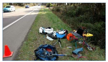
and marine soil, and rock properties that are very difficult to obtain through alternative methods. SA recorded passive ambient vibrations (background noise) augmented by an active, un-timed seismic source (plate and hammer) operated along the array to induce higher frequency, rapidly attenuating energy.
