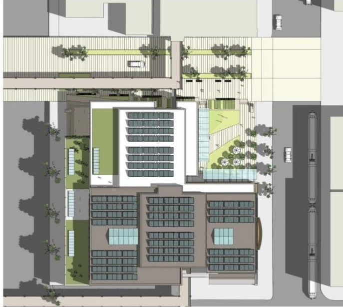
VIEW OF ROOF AND SITE The roof space will be covered with mechanical equipment penthouses, photovoltaic panels, skylights, and greenroofs, as appropriate. This illustration indicates potential uses for the roof which will be further developed in Schematic Design.
