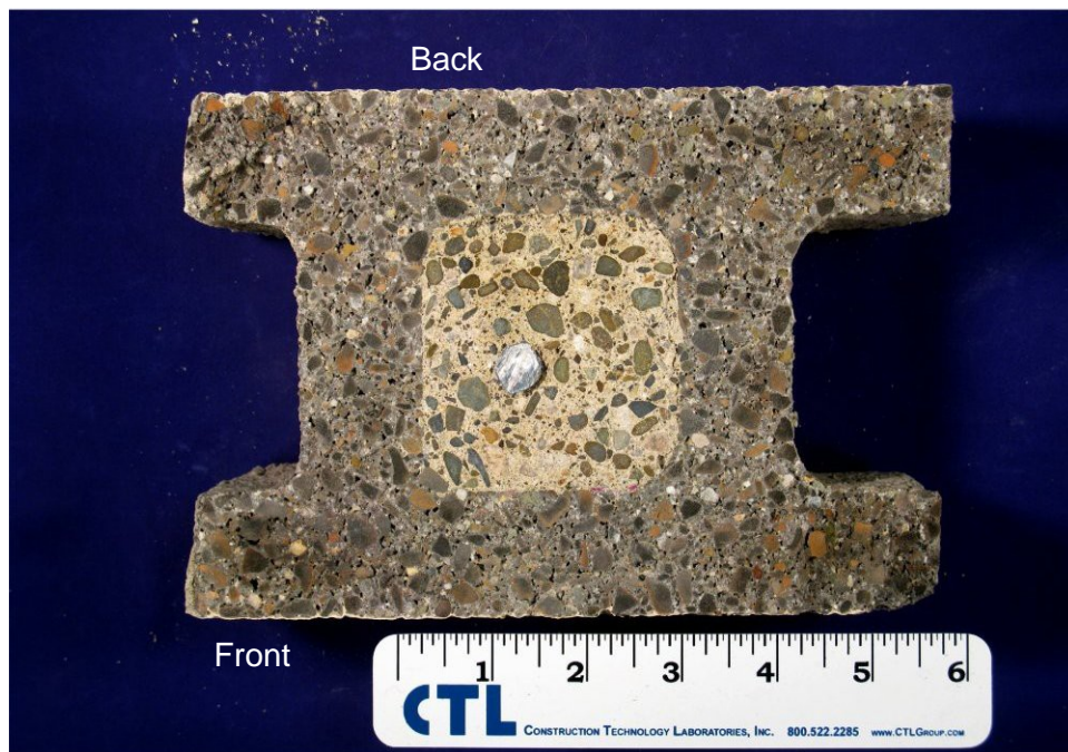
4b. Sample INTERIOR. No cracks are observed.
