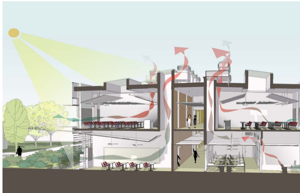
Figure 14: Schematic of a Naturally Ventilated Building
