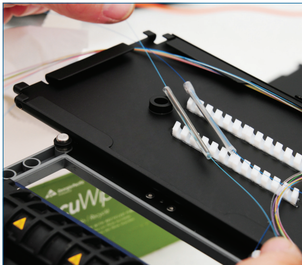
Splice Tray Installation with Gel-Sealed End Cap | Photo LAN4737
