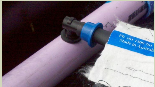
Figure 5.4.5: KISSS BFF 90° Ring-Lock Start Connector with KISSS BFF Material. Notice that KISSS drip tape is protruding out from under the fitting's blue compression ring.
