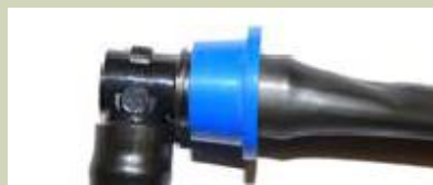
Figure 5.4.2: Insert the drip tape over the black part of the fitting, under the blue compression ring. Push drip tape to the back of the fitting.
