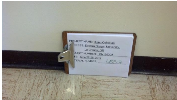
Photograph 15: Lead-containing paint (0.019% lead) was identified in the paint sample LBP-7 obtained from the beige wall paint located throughout the building.
