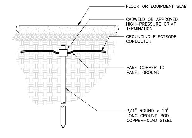
A. GROUND ROD MUST BE INSTALLED IN DIRT NOT IN GRAVEL.
