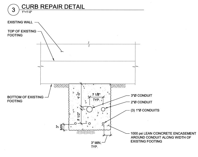
4 CONDUIT ENCASEMENT DETAIL AT EXISTING FOOTING
