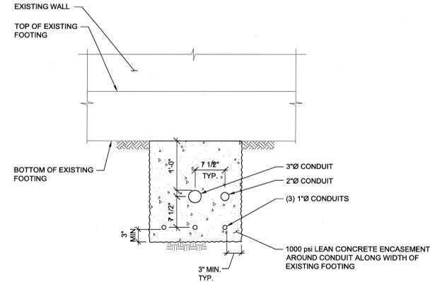
4 CONDUIT ENCASEMENT DETAIL AT EXISTING FOOTING
