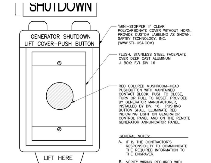
**GENERATOR EMERGENCY REMOTE POWER SHUT-OFF**
