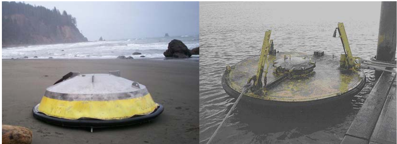
Figure 21. NDBC Buoy 46029 (Left) and 46050 (Right) after they broke free during the Great Coastal Gale of 2007 (Figure reproduced from NDBC, 2008).
