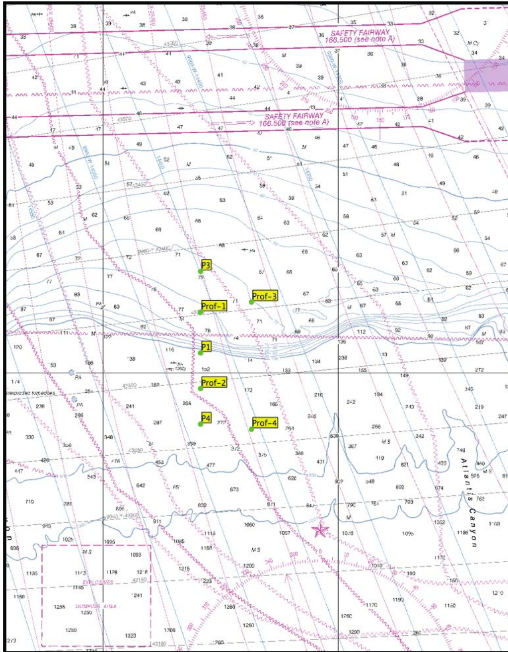
Figure 24. Pioneer moored array area from NOAA nautical chart 12300. Note the explosives dumping area in the lower left-hand corner. Squiggly lines mark submarine cables. Green dots are initial Pioneer mooring sites.
